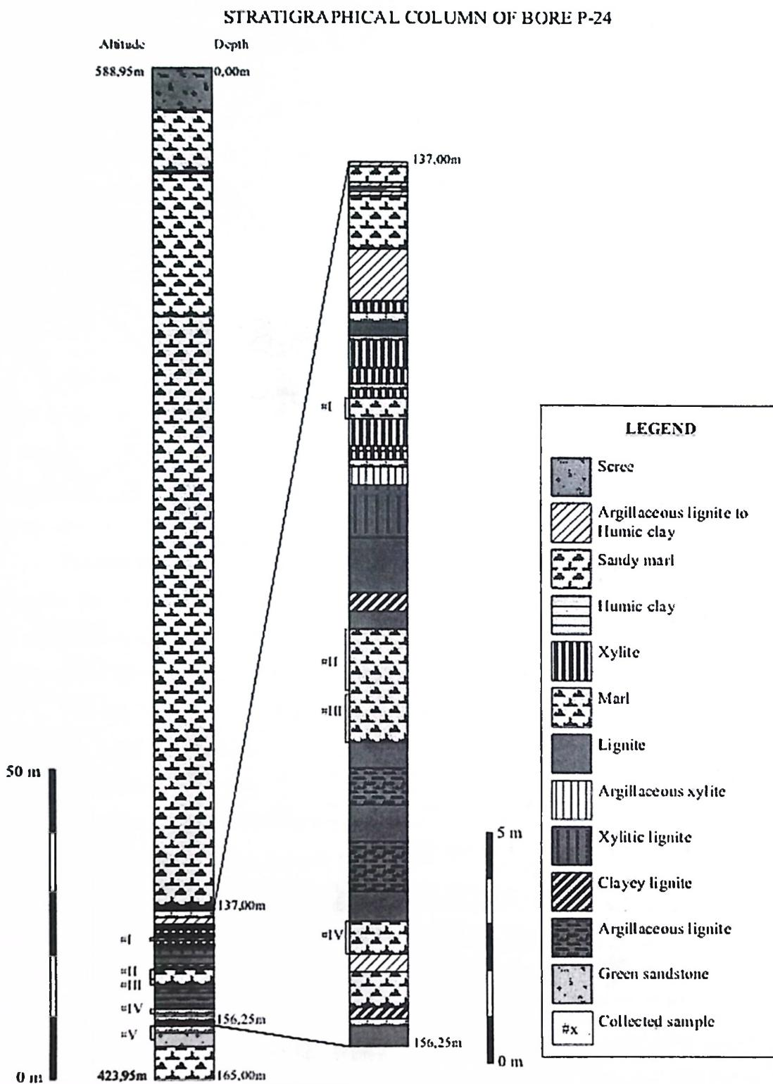
**Figure 2: Stratigraphical column of bore P-24**
