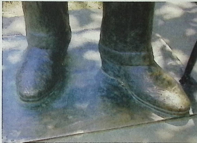
Fig. 9. Removal of "patina" on feet of the statue.
