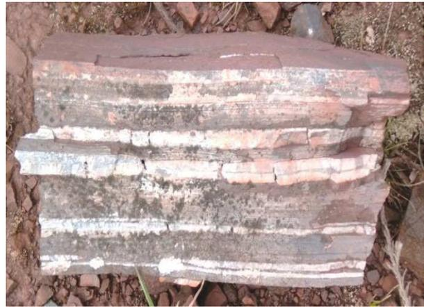
**Fig. 2:** Sample of BIF deposition at Ngwenya (length of the sample about 24 cm).
