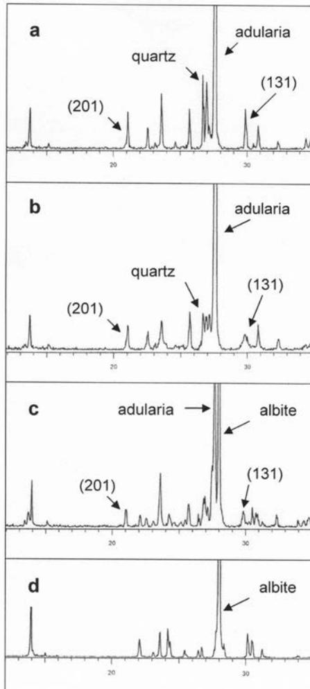
**Fig. 2.** X-ray powder diffraction diagrams of various Greek adularia and albite. a) adularia from a paragneiss-hosted fissure (Thassos Island); b) adularia with green-colored quartz containing byssolith inclusions from orthogneiss-hosted fissure (central Evia); Adularia and albite from orthogneiss-hosted fissure (central Evia) d) transparent albite from a pegmatoid (central Evia)
