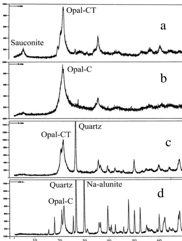
**Fig. 2.** X-ray powder diffraction diagrams of various Greek opals (a): green opal-CT (color due to sauconite admixtures) from Sapes; (b, c) white and brown opal-CT and quartz from Lykofi Evros; (d) opal-C, quartz and alunite from Limnos Island.
